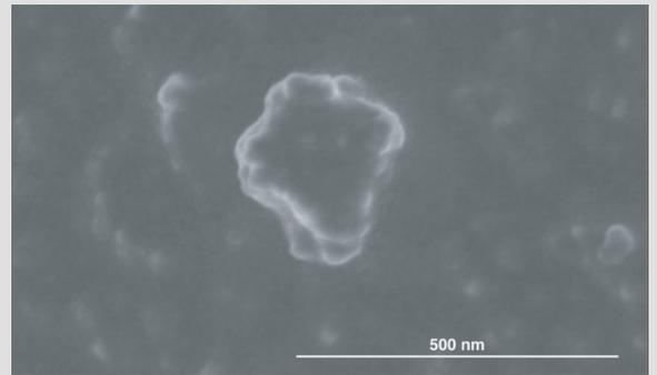
The CO<sub>2</sub> converts into nano-sized minerals, as seen in this Scanning Electron Micro-graph image.
