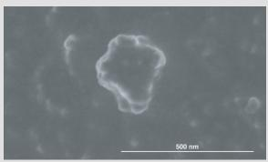
The CO<sub>2</sub> converts into nano-sized minerals, as seen in this Scanning Electron Micro-graph image.
