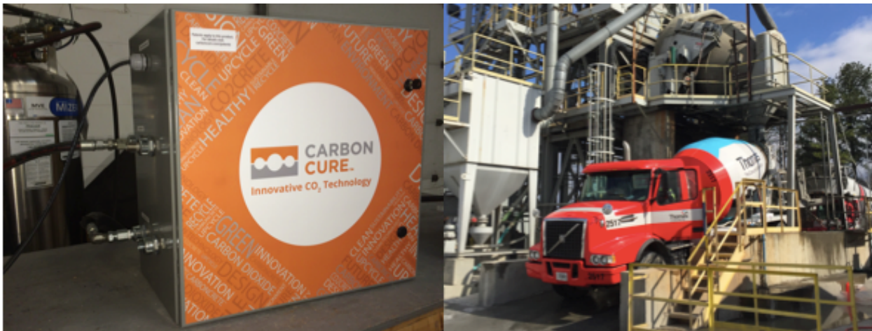
The CarbonCure CO 2 recycling technology (left) has been installed at the Thomas Concrete Doraville plant (right).
